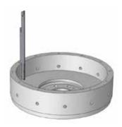
For correct clutch operation on a 14" pot style flywheel this dimension must be 2.937". When resurfacing these flywheels you must take the same amount from the clutch mounting surface as you do the friction surface to maintain 2.937".
